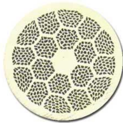
Figure 5.3 Example BSCCO Multifilament Round Wire in Ag Stabilizer (Graphic provided courtesy of Oxford Instruments)
